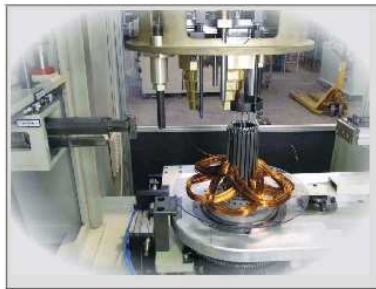
COIL WINDING UNIT
